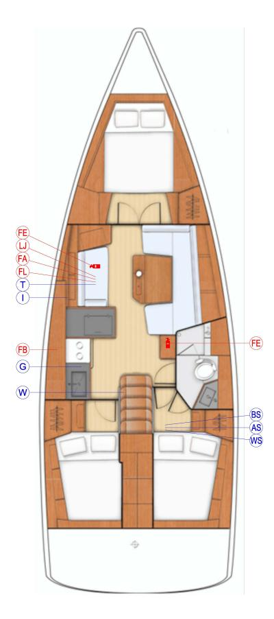
Construction year: 2020 Length: 12.4 m Beam: 4.2 m Draft: 2.2 m Fuel capacity: 195 | Water capacity: 530 I - Tank 1: 330 I - Tank 2: 200 I
