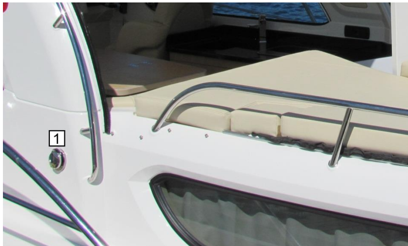
Picture 46: The shore connection (1)
