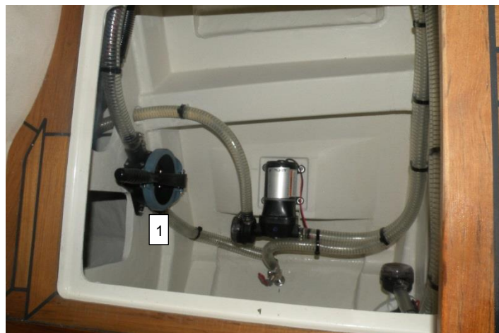
Picture 19: Location of the manual lensing pump in the front cabin area (1)
