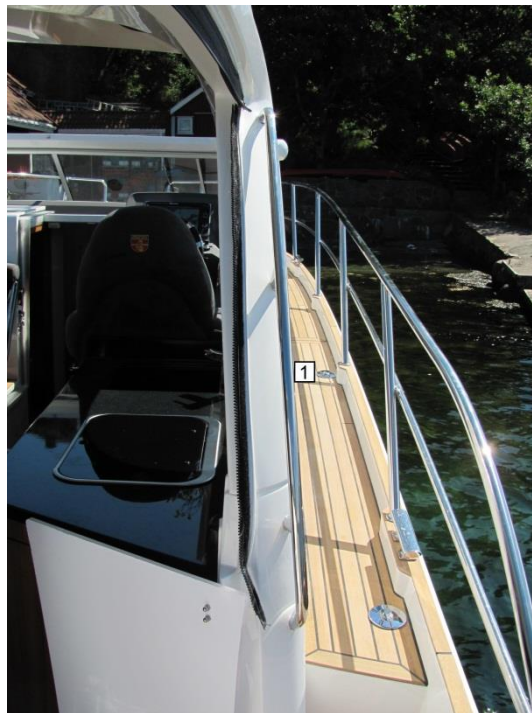
Picture 49: Location of deck discharge (1)
