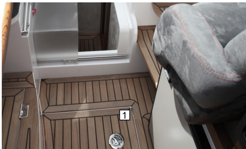
Picture 17: Cockpit drain in the engine hatch canal – starboard side (1)
