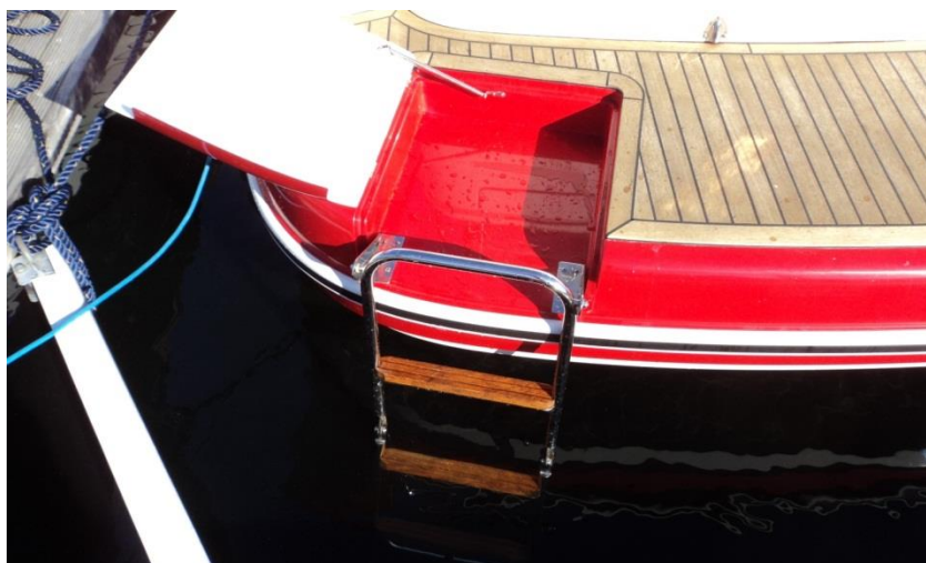
Picture 15: Bathing platform with open ladder cover
