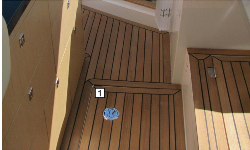
Picture 18: Cockpit drain in the engine hatch canal – port side (1)
