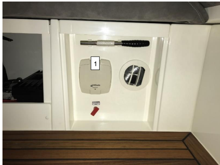
Picture 20: Location of the second manual pump (1) (under the sitting group bench)
