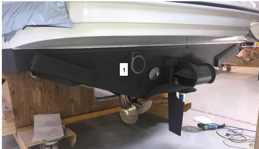
Picture 33: The exhaust hose is going out under the bathing platform (1)
