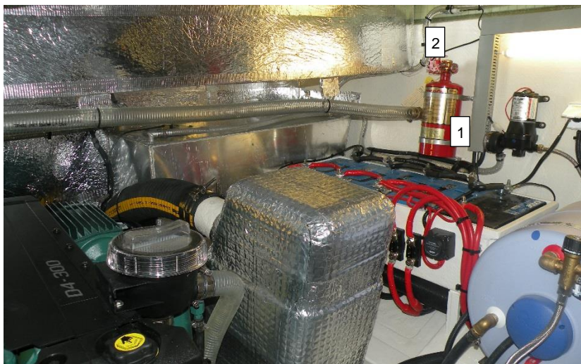
Picture 4: Automatic fire extinguishing system in the engine room (1), fire extinguisher volume level (2)
